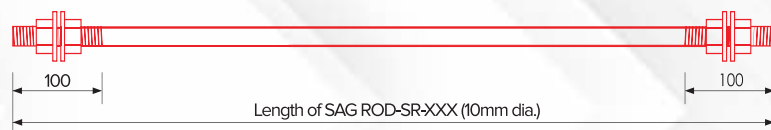
SAG-ROD DETAIL (with four nut & four washers)
